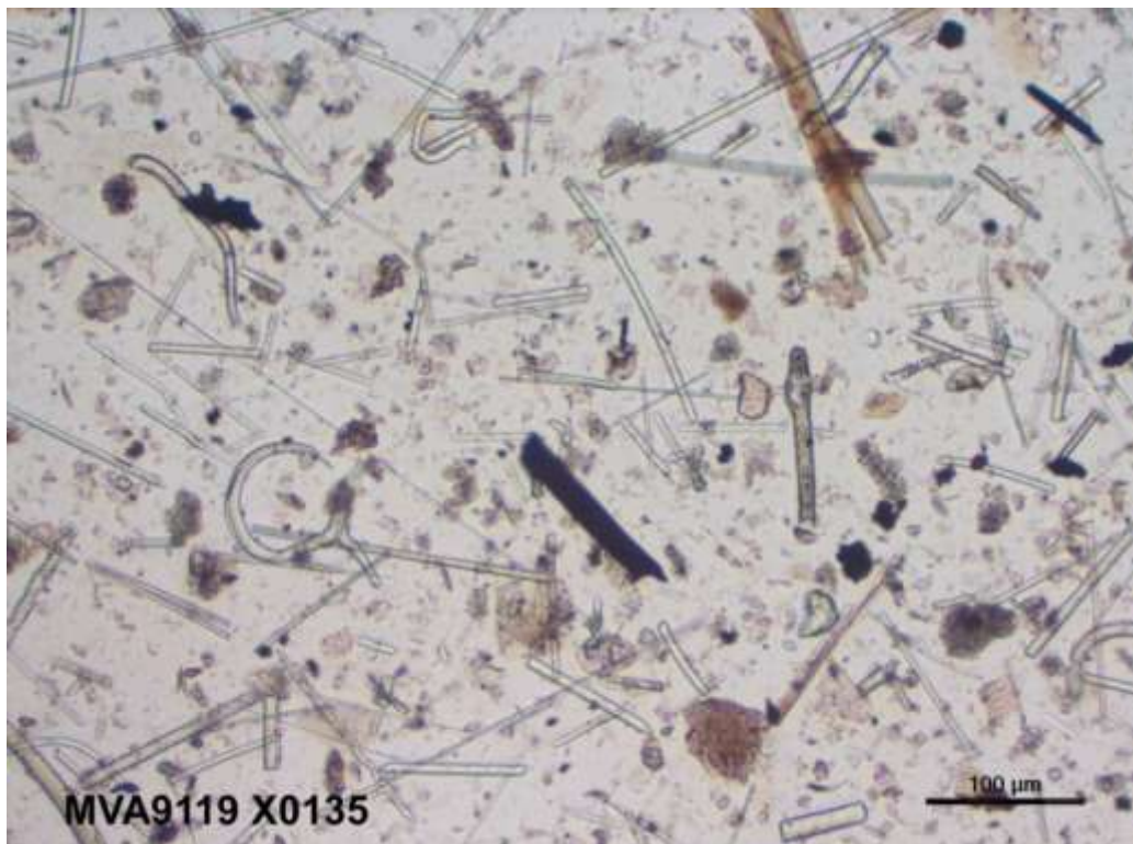
WTC dust as seen with PLM showing common components of glass fibers, cementitious material and soot. Sample X0135, 33 Maiden Ln.
